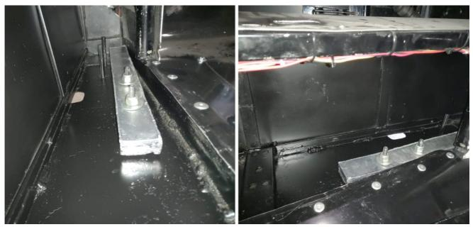
**4\_1\_22** Battery: The position of the car battery cannot be modified from the original manufacturer's positioning, held in place by the appropriate bracket. The use of lighter competition batteries may be accepted including commercial "LITHIUM-ION". Other exotic types, or self-constructed, will not be accepted.
